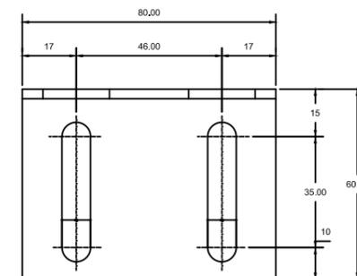
DETALLE DE PIEZA DE ANCLAJE
